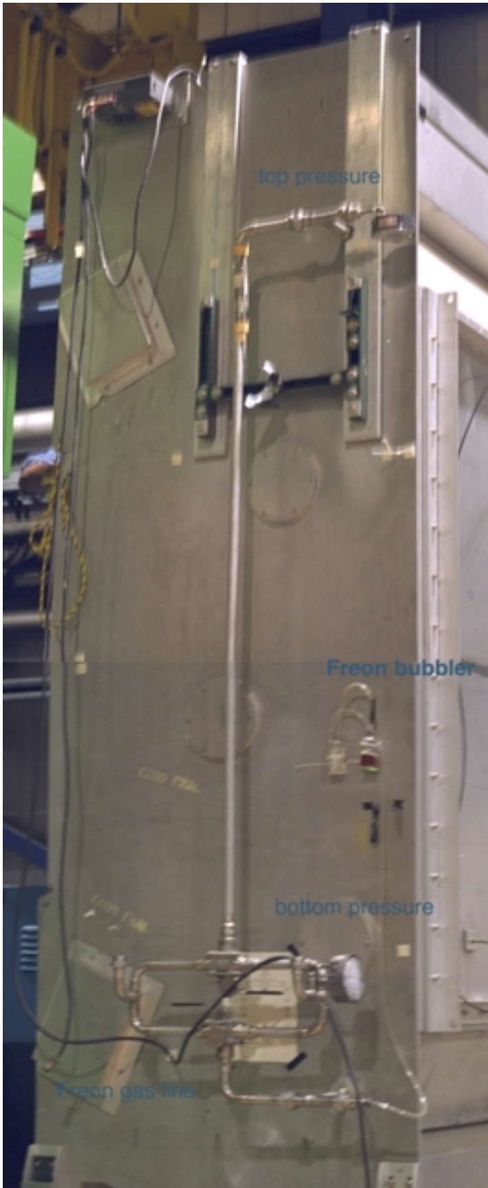
Figure 17. The E690 gas system (composite picture). The Freon pressure at the top and bottom of the vessel are measured by the two helix pressure gauges noted on either side of the stainless steel tubing. The original E766 plumbing system was made of white PVC tubing, which was found to be translucent (causing greatly increased noise rates in pmt's near the gas inlets). The Freon is supplied via the small black tube at the bottom of the counter. A bubbler/barometer allows the gas level to be detected within the vessel providing a check on the fill progress, and the level of the gas when full (but leaking). The two valves seen at the bottom of the counter allow the fill to occur either at the bottom of the vessel, as is the case on the original fill, or at the top of the counter, which is the "top off" mode. E895 added a large bladder at the top of the counter, which was partially filled and allowed the atmospheric pressure to change without emptying and filling the counter. The new back window and the addition of the bladder should make one fill possible, with no additional Freon required for the run.
