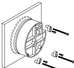
Provide a 4-9/16" dia. opening in panel. Insert gage and secure in place with No. 6-32 machine screws of appropriate length, with adapters, firmly secured in place. To mount gage on 1-1/4"-2" pipe, order optional A-610 pipe mounting kit.
